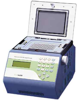
(2003) MyGenie96 Gradient Thermal Block 96웰 형식의 PCR Thermal Cycler
